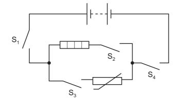
Which three switches must be closed for the heater to work?
