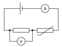
What happens to the readings on the voltmeter and on the ammeter when the temperature of the thermistor increases?
