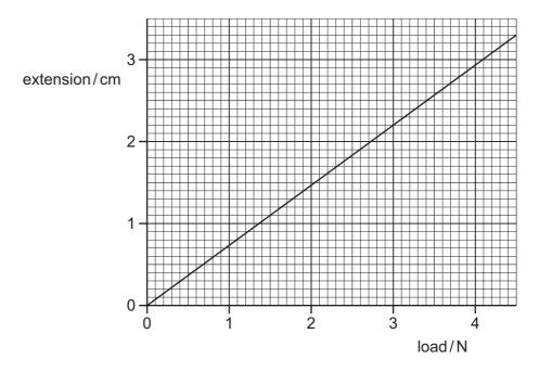
When an object is suspended from the spring, the length of the spring is 19.2 cm. What is the weight of the object?
