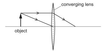
An image of the object is formed on a screen to the right of the lens.
